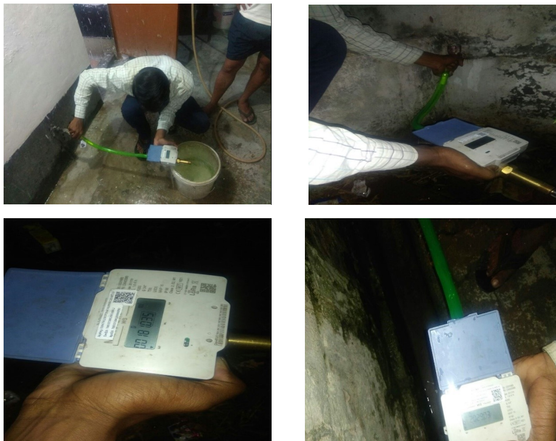
Figure 54: Ultrasonic based consumer meter measurement method of Volumetric Flow Measurements
