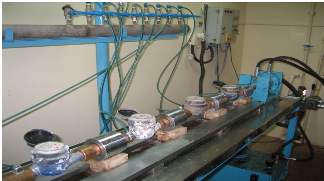
Figure 82: Consumer meter test bench
